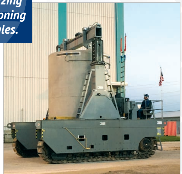
Transport of the 24th MAGNASTOR system to the Kewaunee ISFSI pad.
