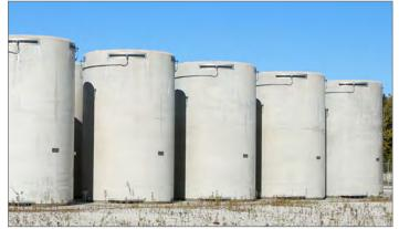
MAGNASTOR: less fuel tube metal, thus lighter and more suitable for lower crane capacities and existing layouts.
