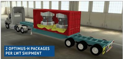
OPTIMUS shipping casks are designed to support legal weight truck (LWT) shipments of a wide range of wastes and fissile material contents in multiple transport configurations.
