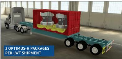
OPTIMUS shipping casks are designed to support legal weight truck (LWT) shipments of a wide range of wastes and fissile material contents in multiple transport configurations.
