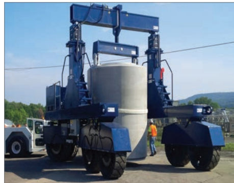
Top photo: 56 loaded NAC WVDP cask systems on West Valley storage pad. Right Photo: NAC WVDP storage cask being moved to storage pad
